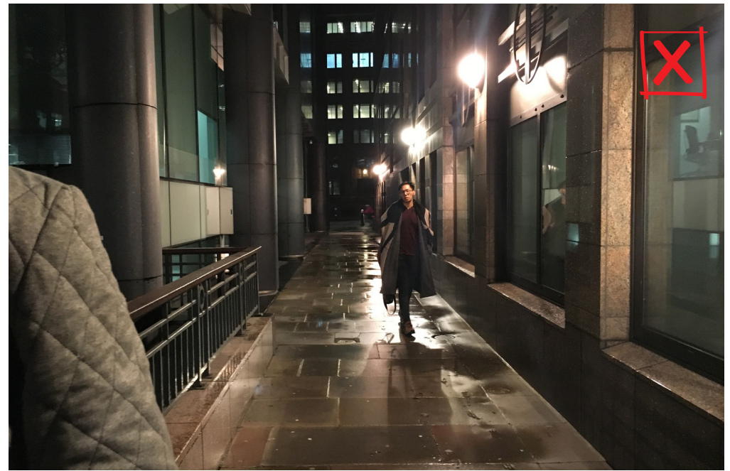
Example of high glare luminaires reducing eye adaptation to lower light levels
